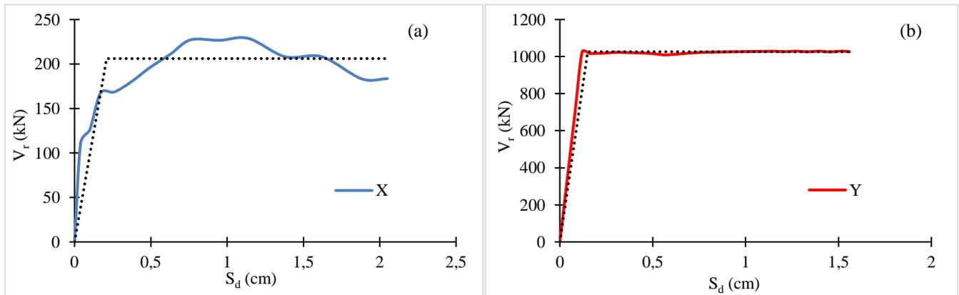
Figure 5: Capacity curves of the stone masonry building: (a) in X direction, (a) in Y direction
