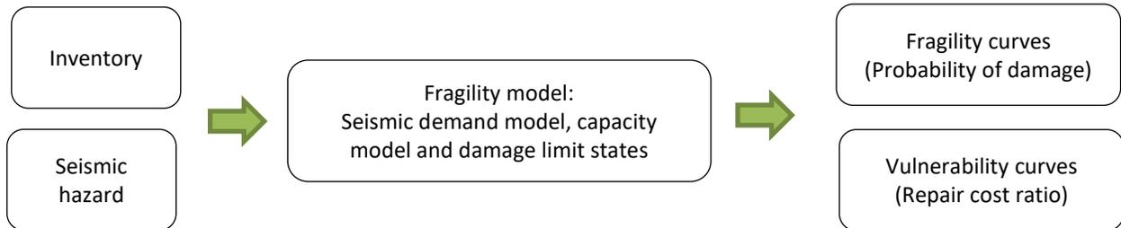
Figure 3: Process of analytical fragility and vulnerability modelling
