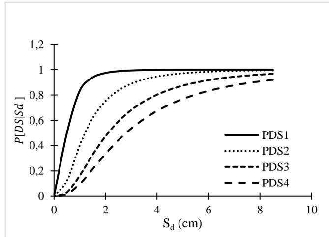
Figure 7: Fragility curves for the prototype stone masonry building
