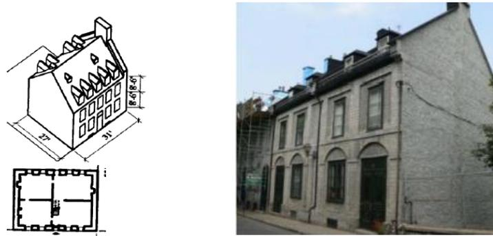
Figure 1: stone masonry building typology in Old Quebec City
