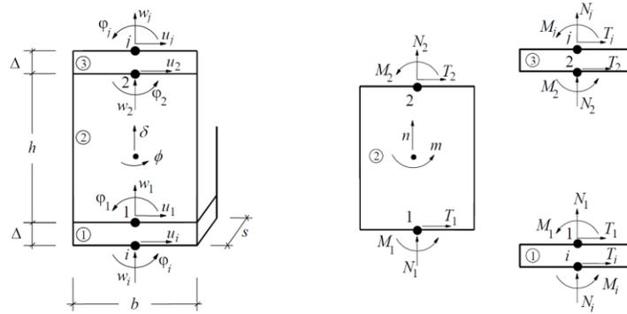
Figure 2: Kinematic model for the macro-element in 3-Muri © [11]
