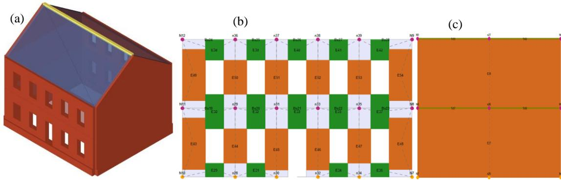
Figure 4: Numerical model of the selected building generated with 3-Muri© software: (a) 3-dimensionel modelling of the building, (b) Discretization of the facade element and (c) Discretization of the lateral firewall
